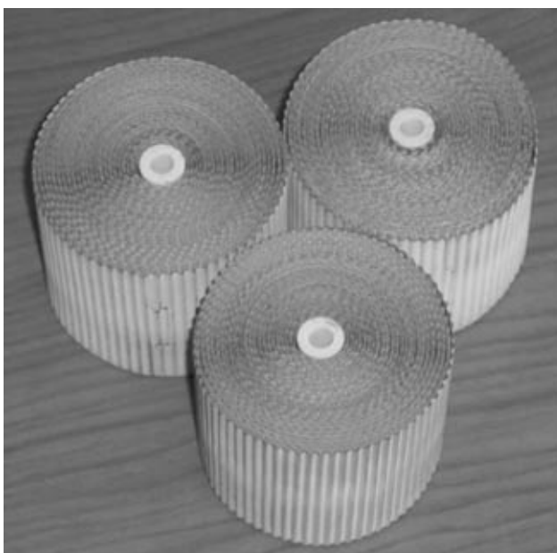
Fig. 33. Typical view of monolith supports based on foils of a thermally stable alloy.
